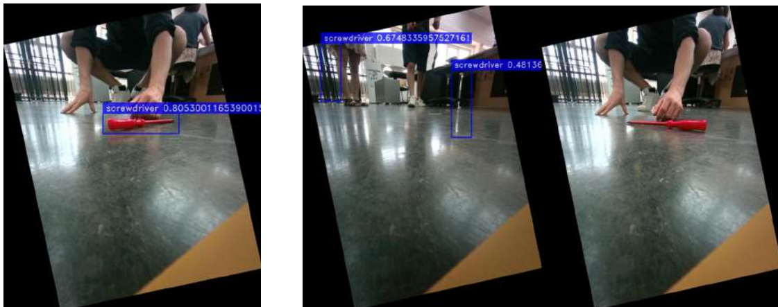
((a)) Detection on a screwdriver with 80.5% confidence.
