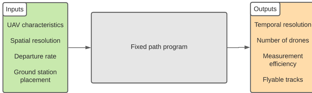
Figure 2.10: Inputs and outputs of fixed path program
