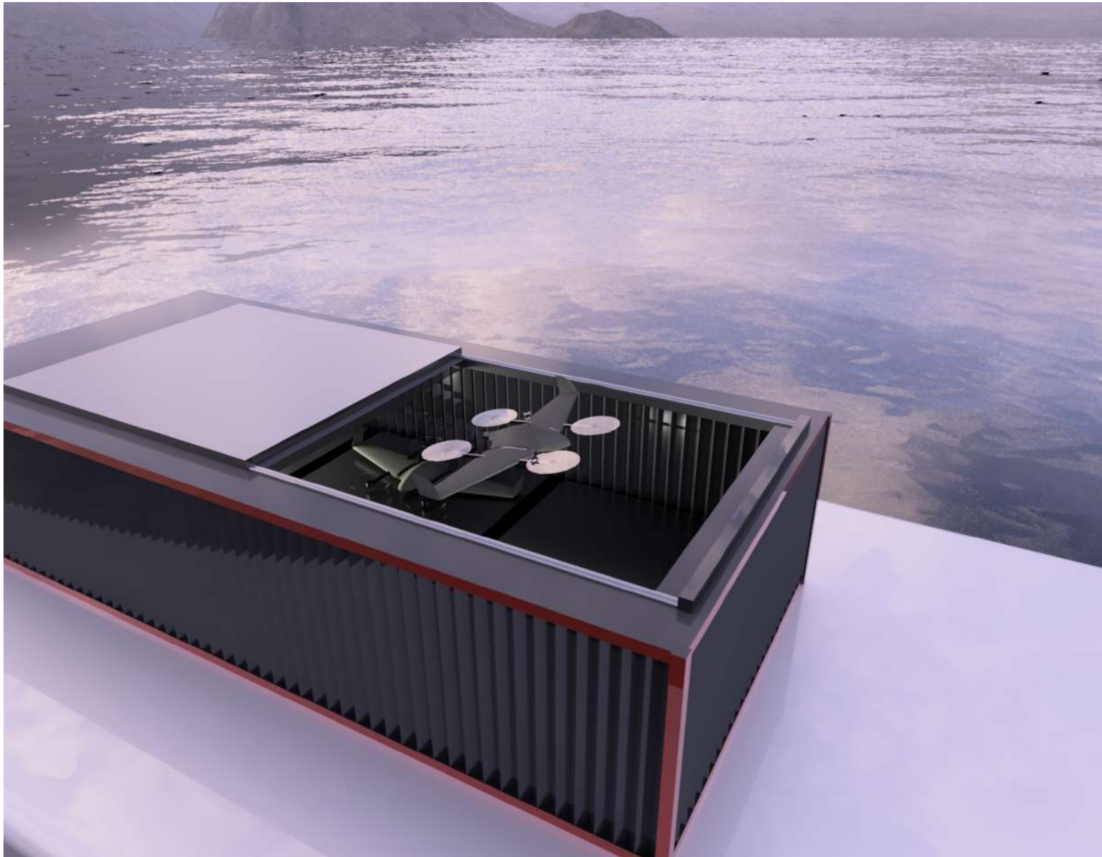
Figure 4.2: Render of the drone storage ground station
